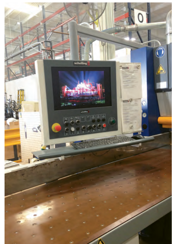
A state-of-the-art control panel on the Schelling FK4, a cut-to-size saw for plastics, is one of the recent additions at General Plastics.
